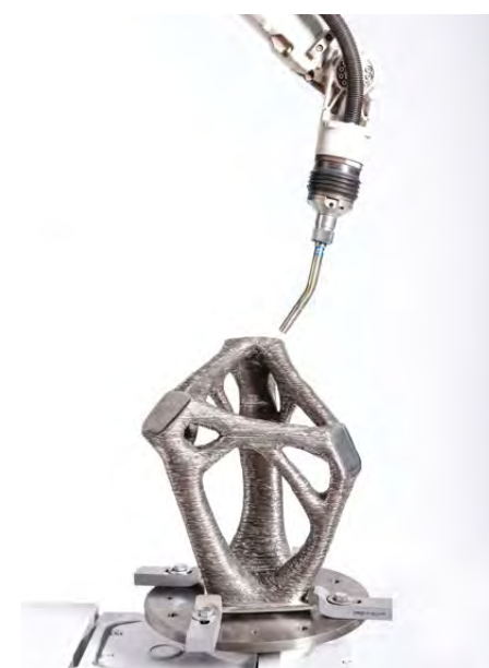
The WAAM-printed structural connector designed by MX3D and Takenaka, made in duplex stainless steel.
