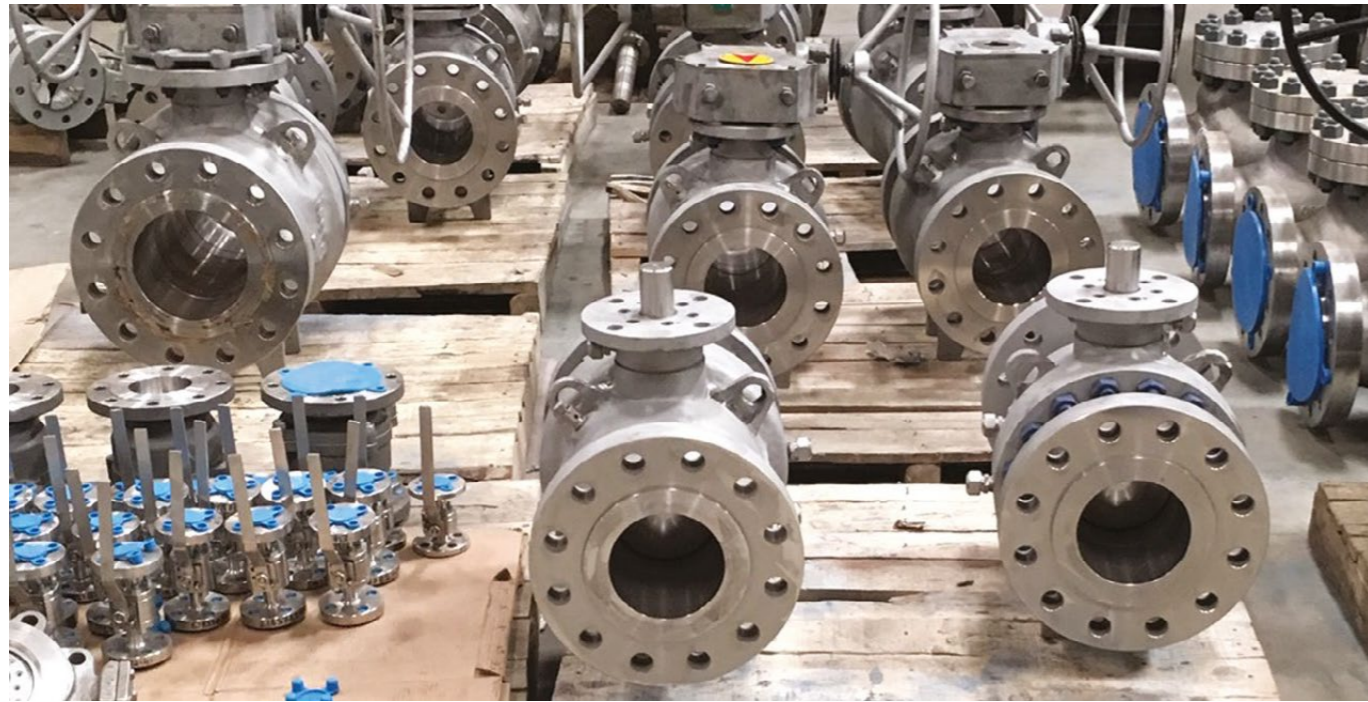
Orseal super-duplex valves are used on FPSOs in the offshore oil & gas industry.
