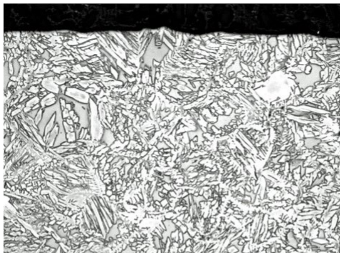
Figure 1. Duplex microstructure with an even mix of austenite and ferrite.
